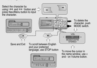
The saved text is displayed during initial loading of disc and at stop mode during play.
